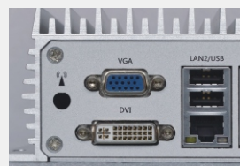
DVI and VGA support asynchronous or synchronous dual display
